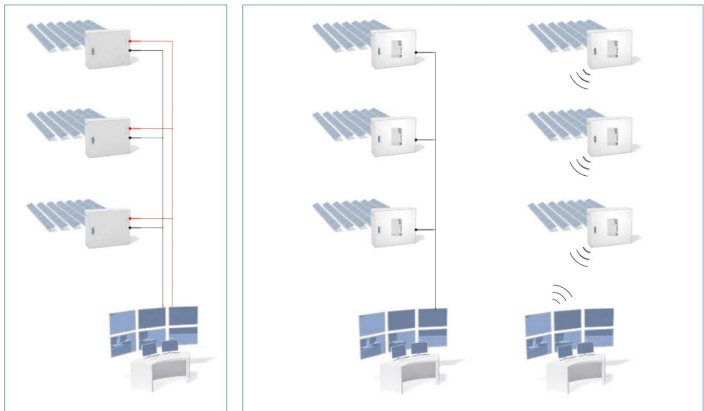
In the application shown, the Combiner Box is connected to a supply line (red, e.g. 230 V AC) and a signal line (black). Laying the lines involves significant installation costs.
